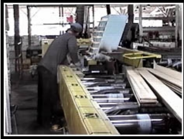
Full guard forces worker to assume extreme trunk flexion to handle bundles.
