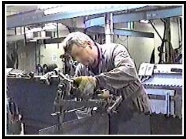
Lowering load away from the body increases the effort in the shoulders and low back.
