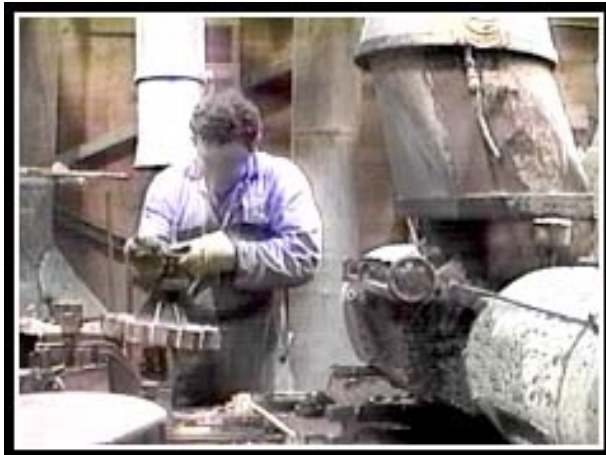
More loading on shoulder and back when reaching into planer to lift side heads
