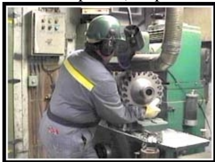
Loading on the back is increased when installing the side head on the grinder this way.
