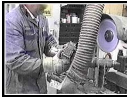
Loading on the back is decreased when installing the side head on the grinder this way.
