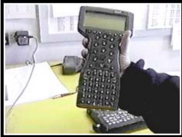
Smaller computer with narrow grip reduces force required to grip and decreases risk of injury.
