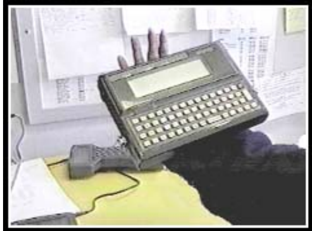
Larger and heavier computer increases the force required to grip and increases risk of injury.
