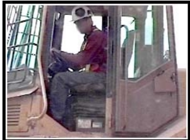
Safer shoulder posture with tilt steering.
