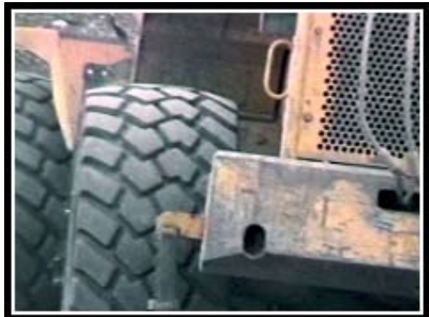
Knobby tires are suitable for softer terrain, where traction is required.
