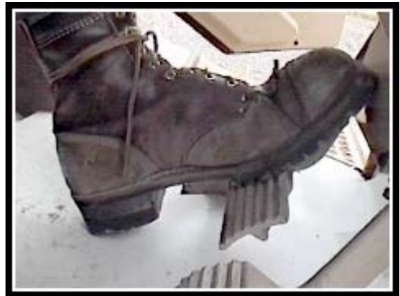
Horizontal foot pedals require less ankle flexion to operate.
