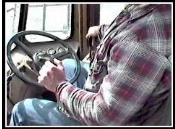
Steering wheel within safer reach envelope.
