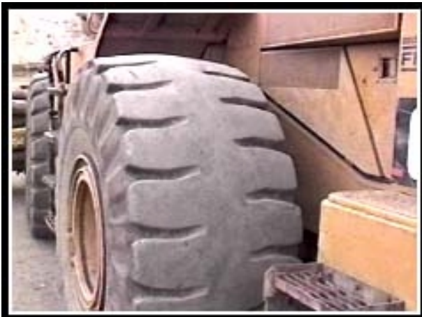
Smooth tires are preferred on hard surfaces to decrease vibration.
