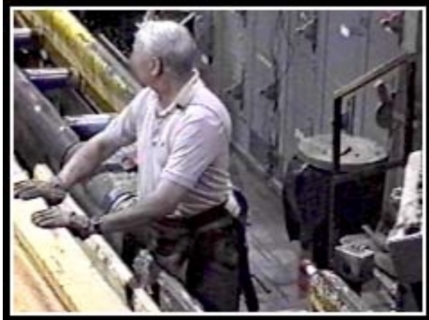
A Horizontal/Vertical Resaw Operator must grip lumber and controls with the wrists bent in order to guide, inspect, and orient it for the saws.
