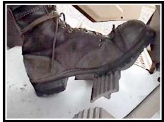
Horizontal foot pedals require less flexion to operate.
