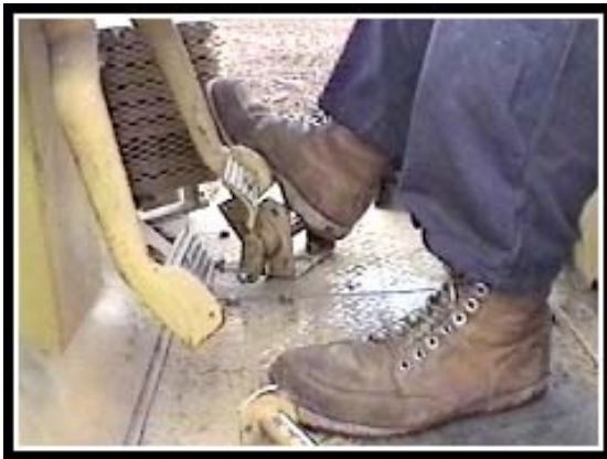
Foot pedals with a vertical surface place more loading on the ankle.
