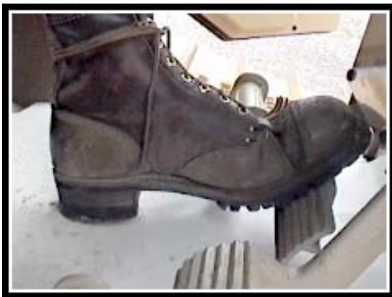
Poor Technique: Using the tip of the foot to activate the foot pedal.
