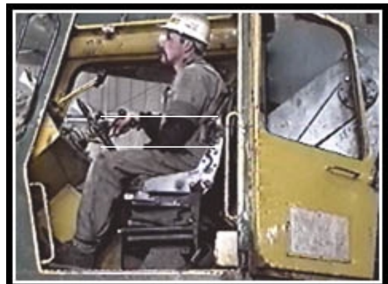
The highest level of operator controls should be located around mid-chest level while sitting down.
