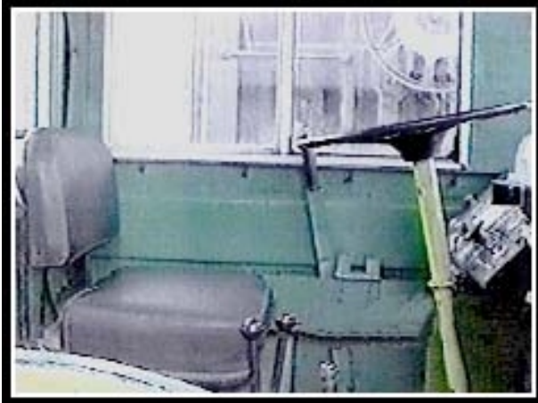
Chairs without good lumbar support. Poorly designed chairs allow the back to lose its natural curve, which increases the risk of injury.
