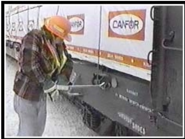
Manually tightening cables using a ratchet.
