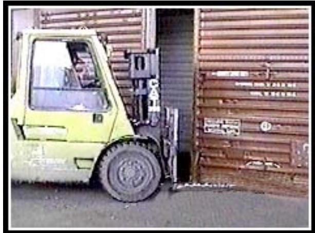
Using forklift to open door.
