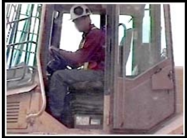
Steering wheel within safer reach envelope.
