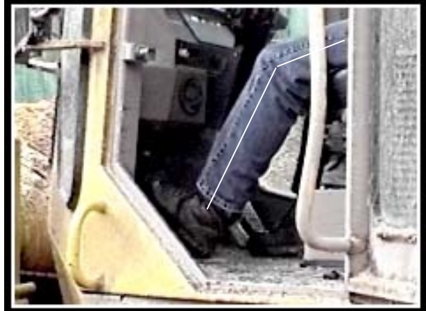
Safer knee position for operating foot pedals.
