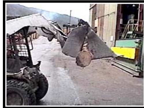
Some Bobcat Operators use a split bucket to handle larger debris.
