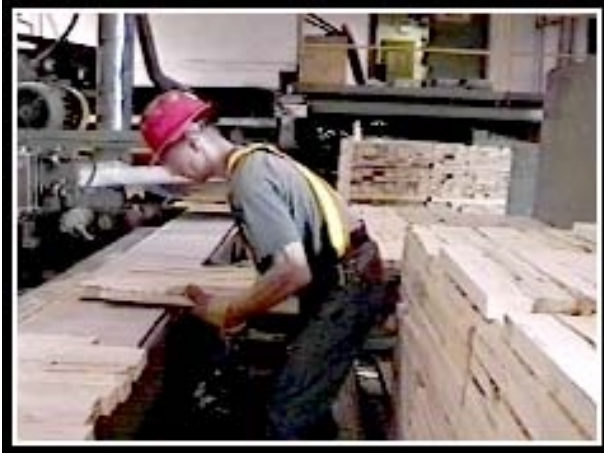
A Block Piler may lift blocks off a conveyor to sort and stack them.
