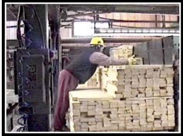
A Block Piler may also bend forward when reaching for blocks on the far side of the conveyor or placing blocks on the back of a load.
